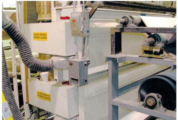
The raw canvas is unwound from a mill roll and passed over a rotating brush to remove foreign objects, while a sanding roller smooths out any unevenness in the weave.
