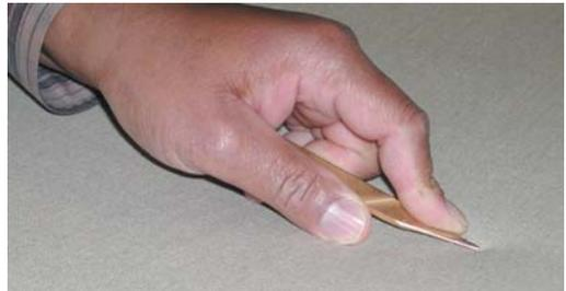
The surface is inspected for weaving imperfections, which are hand picked clean. Aligning the individual yarns closes in any resulting holes.
