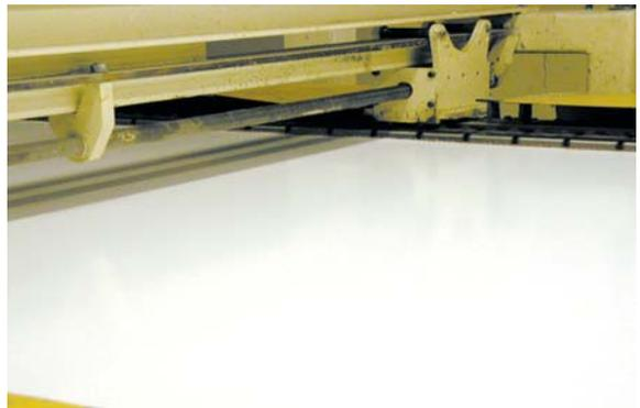
Sizing is applied on the coating table and then metered to the desired coating weight. The canvas is stretched flat and enters the drying chamber.
