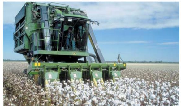
Today, cotton is entirely machine harvested in the U.S. where stripper harvesters remove the cotton boll from the plant.
