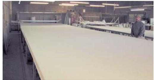
Raw linen is tightly stretched on a frame that exerts a uniform pressure under constant temperature and humidity control.
