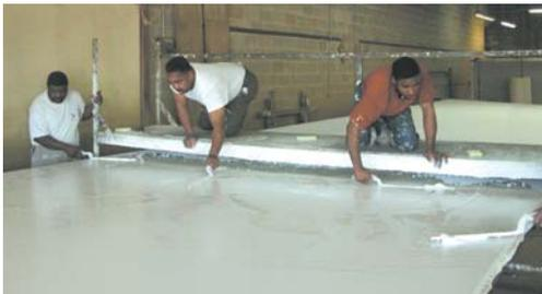
A moving bridge is used to help craftsman reach across the canvas. The horizontal position prevents the sizing from running down vertically and congealing at the bottom.
