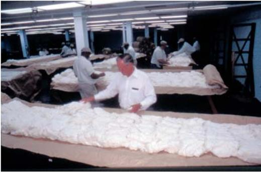
The cotton lint is baled, and classified according to fiber strength, staple length, length uniformity, grade and fineness.
